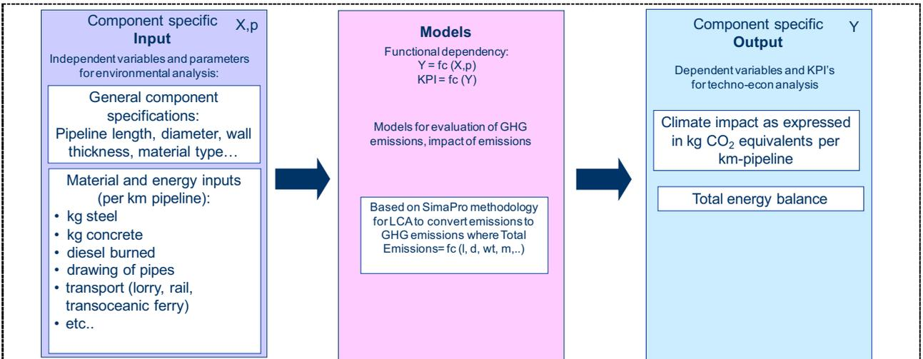
Figure 4: Example for a transport module for environmental assessment of pipeline for CCS.
