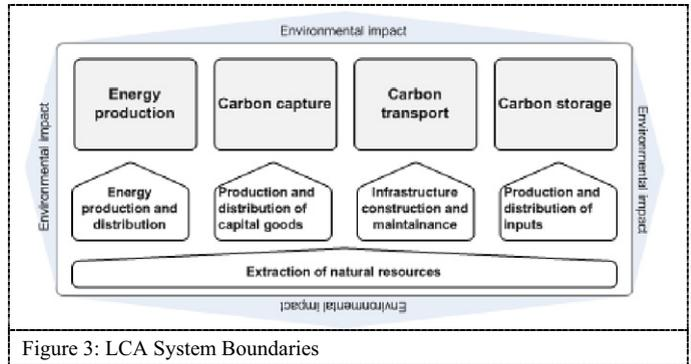
Figure 3: LCA System Boundaries
