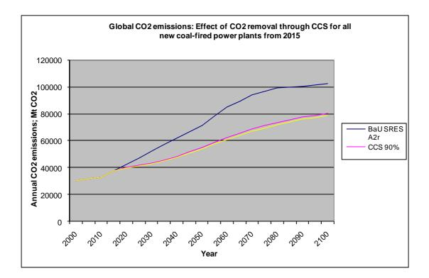
Figure 2. Comparison of global CO<sub>2</sub> emission for the A2r BaU scenario and the CCS scenarios.
