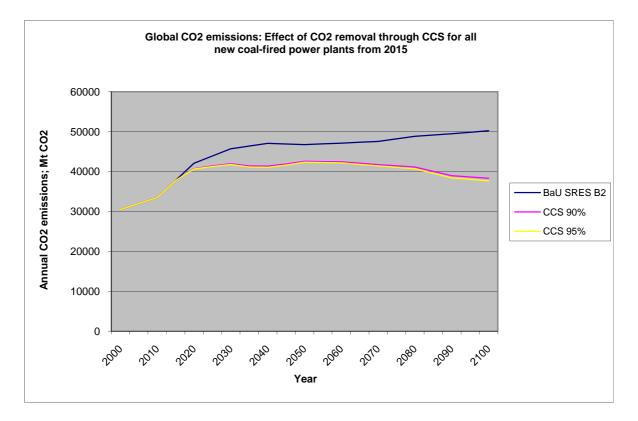
Figure 1. Comparison of global  $\mathrm{CO}_2$  emission for the B2 BaU scenario and the CCS scenarios.
