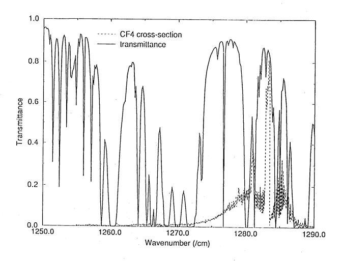
Figure 1: An approximate line-by-line transmittance calculation for a 1 km path at the surface, with typical mid-latitude concentrations, for water vapour (solid line), as a function of wavenumber. The dashed line shows the cross-sections of  $CF_4$ , in relative units, from McDaniel et al. (1991).
