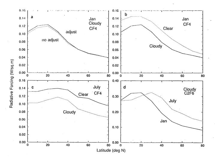
Figure 2: Latitudinal variation of radiative forcing (Wm<sup>-2</sup>) for a 1 ppbv increase in fluorocarbon concentration as calculated with the UoR model. (a)  $CF_4$  forcing with and without stratospheric adjustment for the January cloudy case. (b)  $CF_4$  forcing with and without clouds for January, including stratospheric adjustment. (c) As (b) but for July. (d)  $C_2F_6$  forcing for January and July assuming cloudy skies and including stratospheric adjustment.
